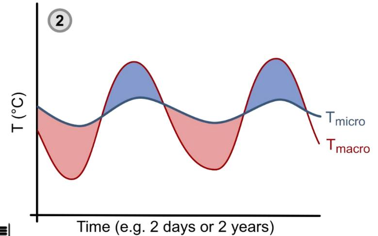
$$\text{Offset} = \text{Temp}_{\text{micro}} - \text{Temp}_{\text{macro}}$$
